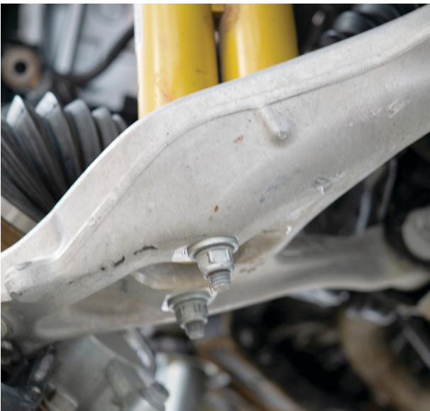
Fig. 9: Take off the bar-pin bolts.
