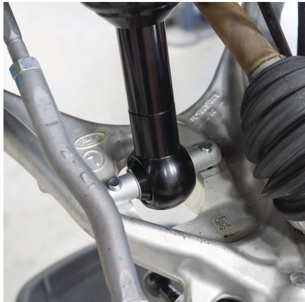
Fig. 13: Fasten the bar-pin bolts.
