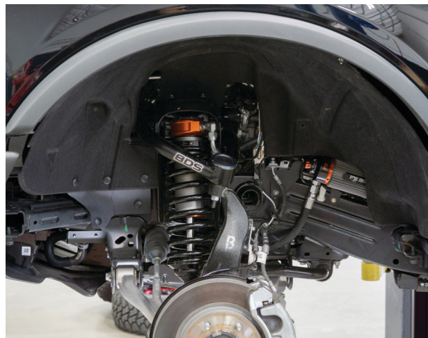
Fig. 29: Trim the fender liner.
