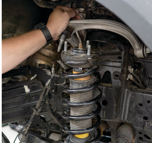
Fig. 8: Free the coil-over from the coil bucket.
