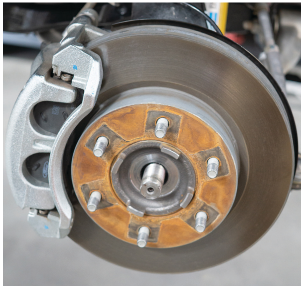
Fig. 5: Push the axle shank flush.
