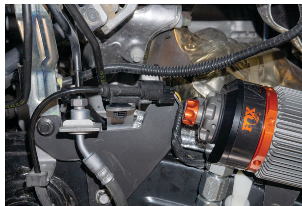
Fig. 27: Fish the ABS wire through the bracket.
