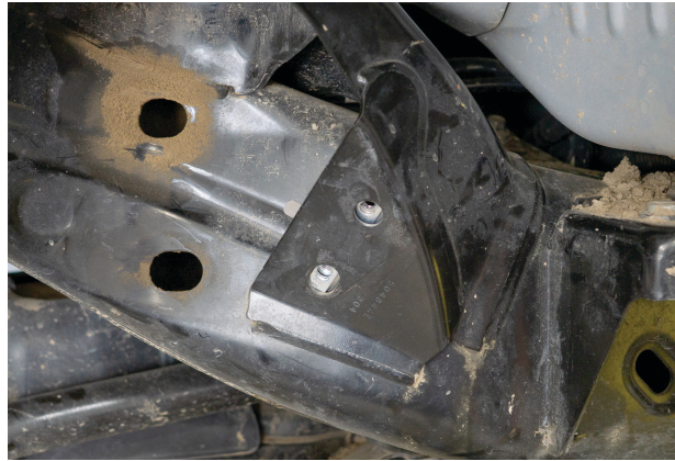
Fig. 45: Locate the backing plate's speed nuts with the holes in the frame.
