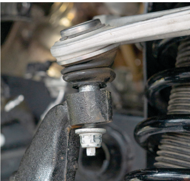
Fig. 6: Separate the UCA from the upright.
