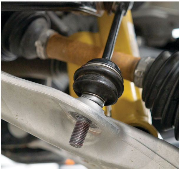
Fig. 4: Disconnect sway bar end link.
