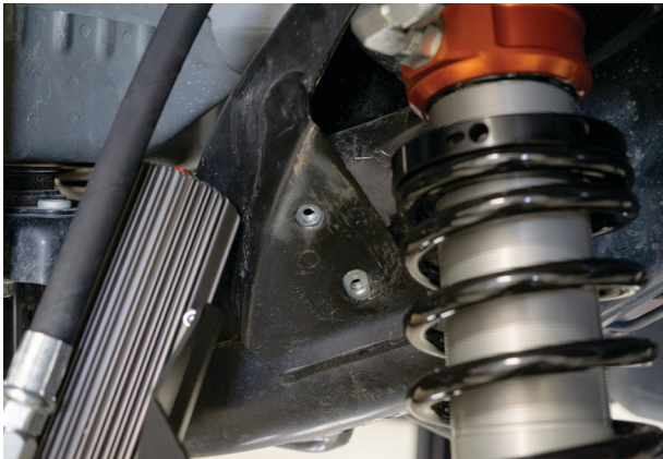
Fig. 46: Align backing plate with the frame.
