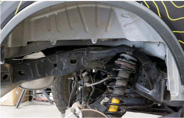
Fig. 343: Pull the fender liner.
