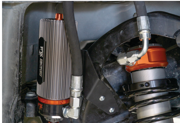
Fig. 47: Mount the reservoir bracket.
