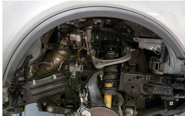
Fig. 1: Pull the fender liner.
