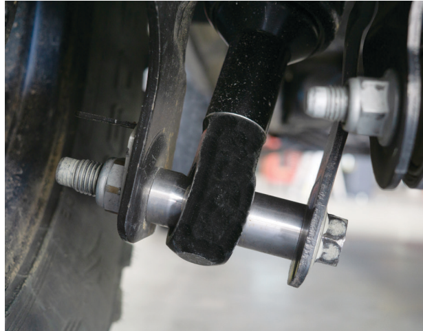
Fig. 41: Note the larger spacer is on the inboard side.
