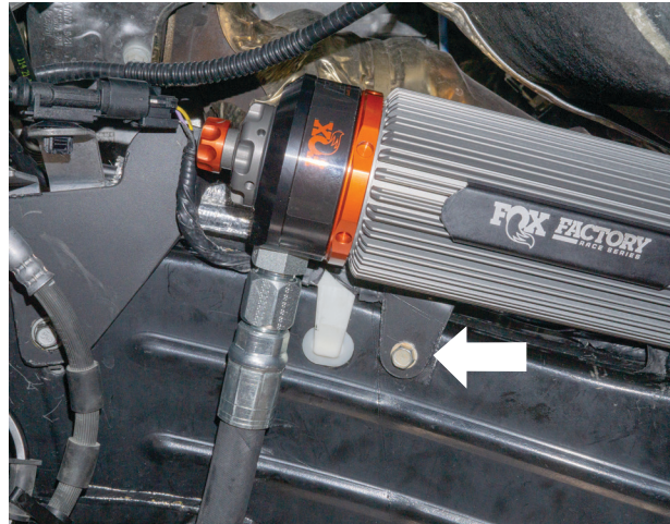
Fig. 28: Install the self-tapping screw.
