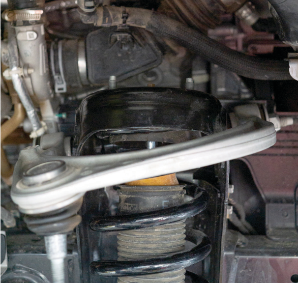
Fig. 7: DO NOT remove the center nut.
