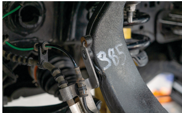
Fig. 2: Disconnect brake line bracket.
