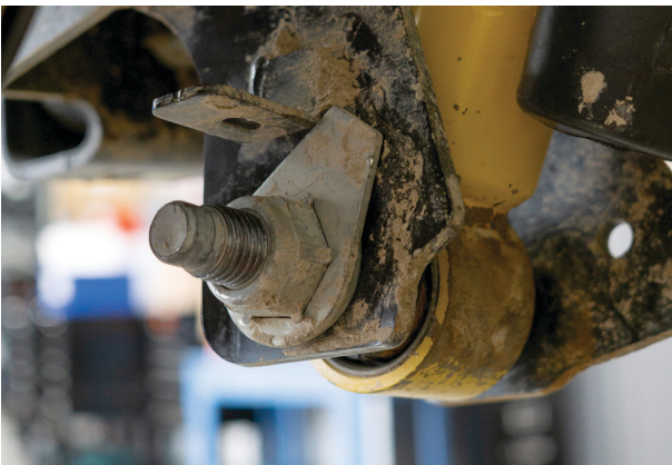
Fig. 36: Loosen the lower mounting bolt.
