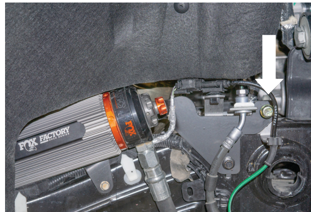
Fig. 25: Install the provided bolt on the passenger side's reservoir bracket.
