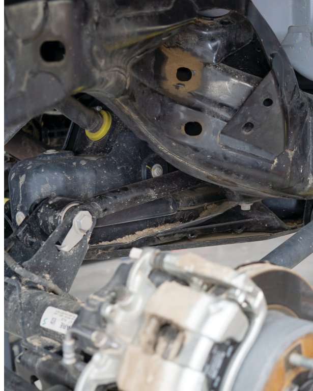
Fig.38: Remove the stock coil-over.
