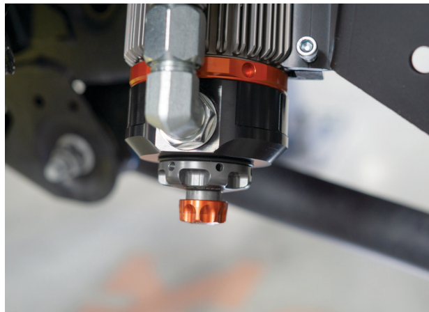
Fig. 43: Mount the reservoir to the bracket.
