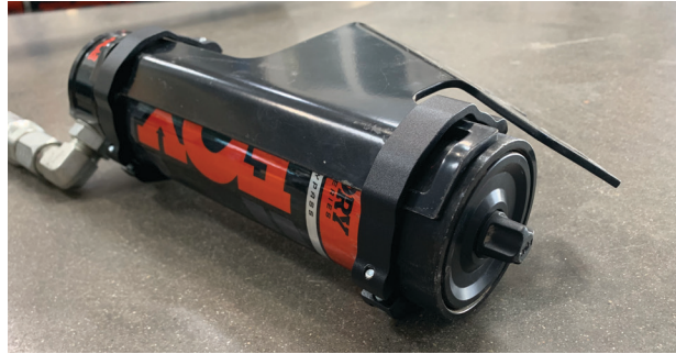
Fig. 5: This image is for informational purposes only to demonstrate how the reservoir brackets should interface with the clamps. Mount Group A and B brackets to the vehicle before you install the reservoir.
