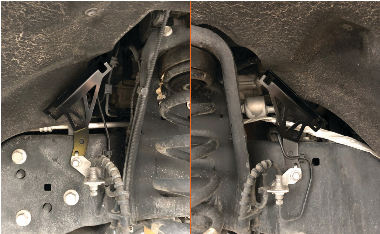
Fig. 3: Align the reservoir bracket with the brake line tab.
