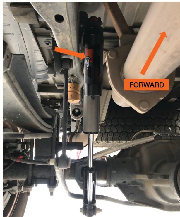
Fig 9: The right side shock must be mounted with the reservoir pointing forward.
