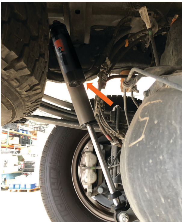
Fig 8: The left side shock must be mounted with the reservoir pointing inward.
