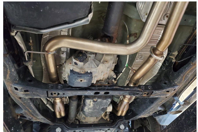
Headers and leads installed
