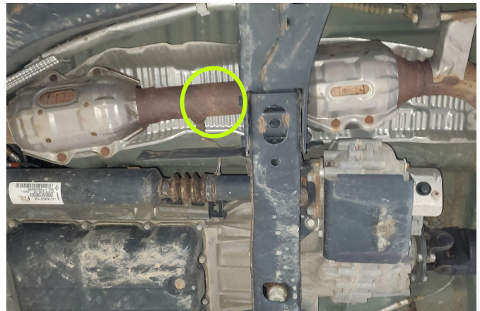
Detail 8: Cut location for driver side catalytic converter pipe.
