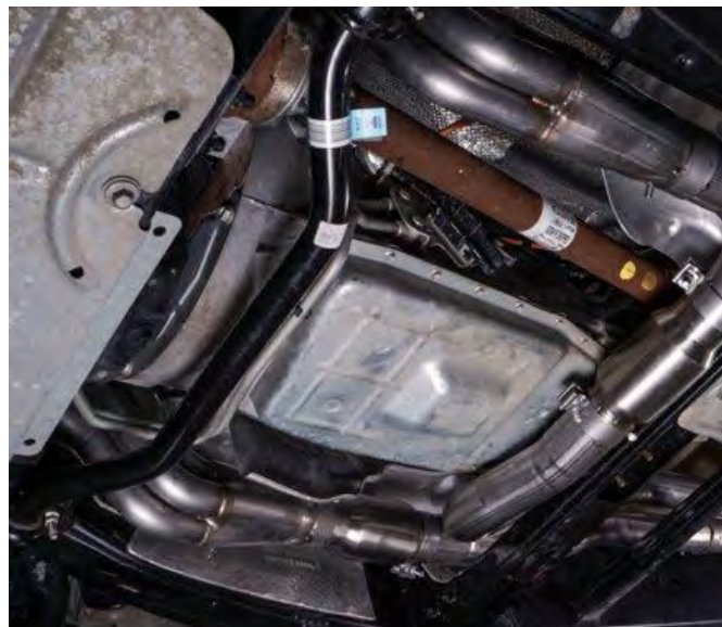
Installed headers close-up
