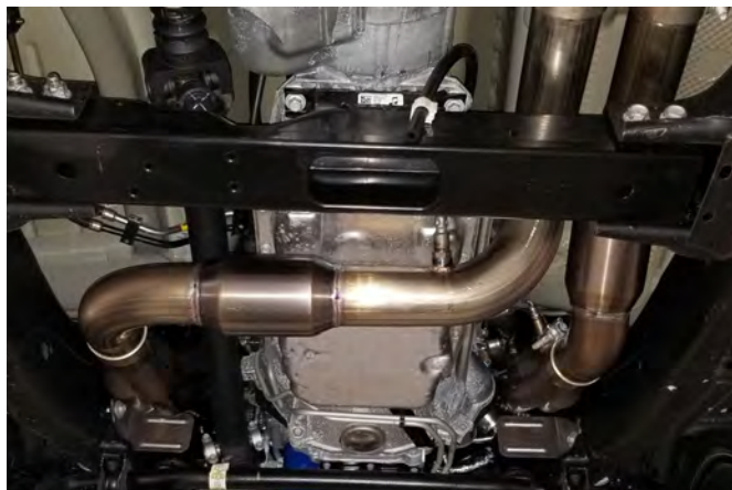
Detail 16: Headers and leads installed
