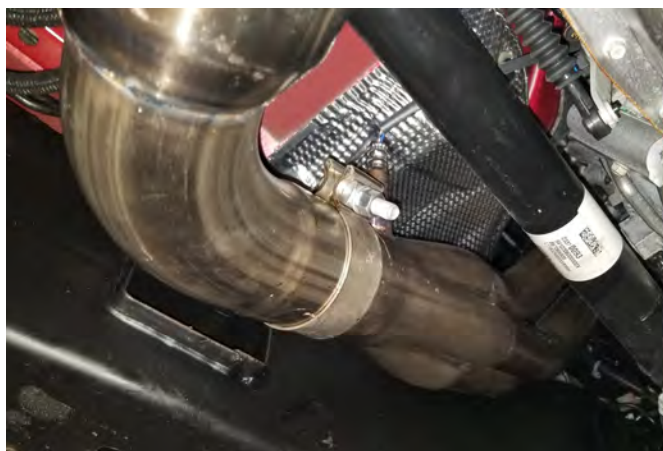
Detail 18: Driver side header - lead pipe connection.
