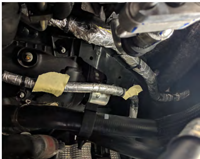
Detail 15: Wire harness to move. Locations for unlooming marked with tape.
