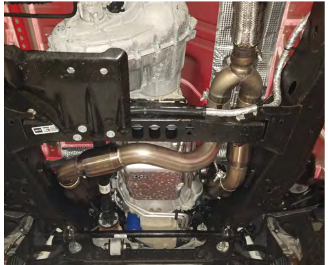
Detail 16: Headers and leads installed
