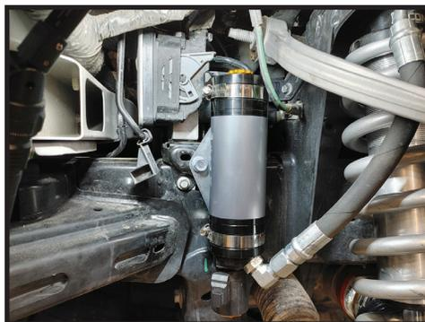
**12.** Passenger side install on 4 cylinder models. Remove the lower rubber fender line and move the fabric liner out of the way. Remove the rear 10mm bolt that holds the heater lines. Place the 2500020 bracket in position and reinstall factory bolt, as shown. Use supplied hose clamps to secure reservoir to brackets. [FIGURE 11 & 12]
