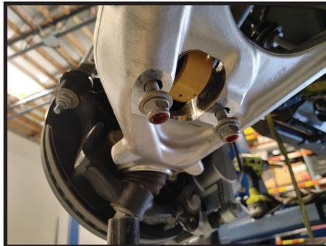
7. Lower the arm down so the coilover can be removed. [FIGURE 6]
