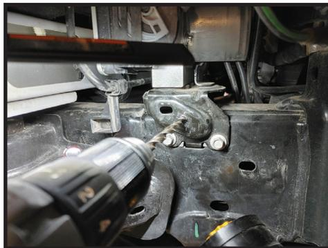
**11.** Install the 250002 bracket as shown using one 3/8" self tapping bolt. [FIGURE 10]
