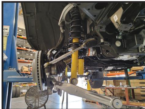
**8.** With the factory coilover removed, install the ICON coilover. Upper mount first using the supplied 3/8-16 x 1.00 GR8 bolts and split lock washers. Torque to 35 ft-lbs using a 9/16. [FIGURE 7]
