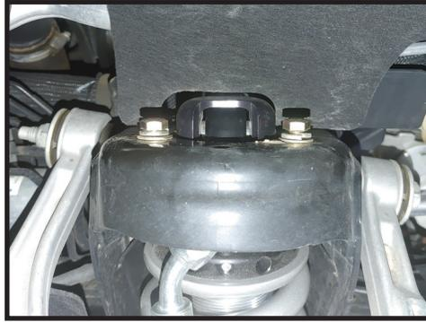
**9.** Reinstall the lower control arm into the frame pockets using factory hardware (snug bolts only) and connect the lower shock to the control arm using the supplied 7/16 bolts and washers. Torque to 70 ft-lbs. Refer to the photo for proper bolt/washer orientation. [FIGURE 8 & 8A]
