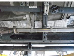
**Step 3:** Begin Installing the new system by attaching Inlet Pipe "A" to the vehicle using the OE Fasteners.
