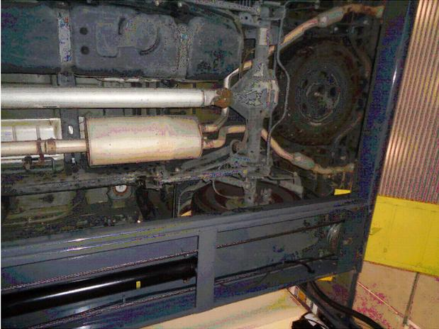
Step 1. Begin removal of the OE muffler by loosening the three clamps attaching the exhaust to OE system. Disengage the hangers from the rubber insulators and remove the muffler. Do not discard or damage the rubber insulators as they will be used to install the new system.
