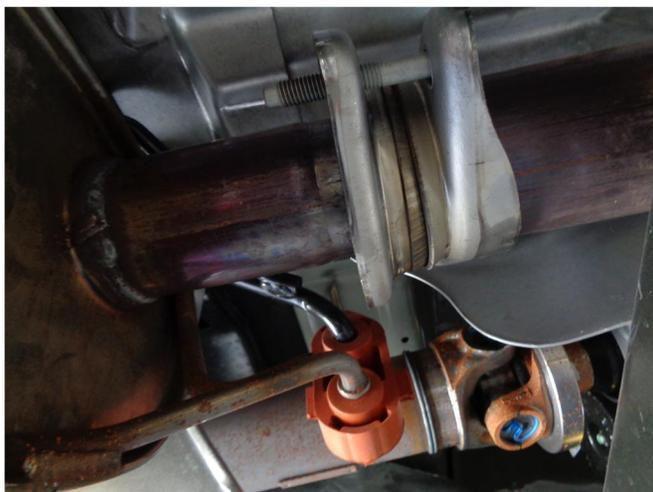
**Step 3.** Unbolt the muffler assembly from the catalytic converter outlet at the flange junction. Disengage all welded hangers from the rubber insulators. The remainder of the system can now be removed.
