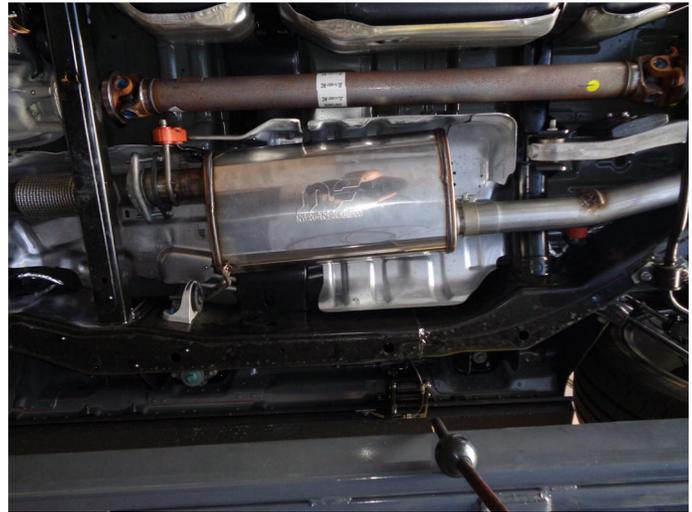
**Step 4.** Begin installing your new MAGNAFLOW system by loosely bolting the Muffler Assembly inlet flange to the flex assembly outlet using the supplied hardware.
