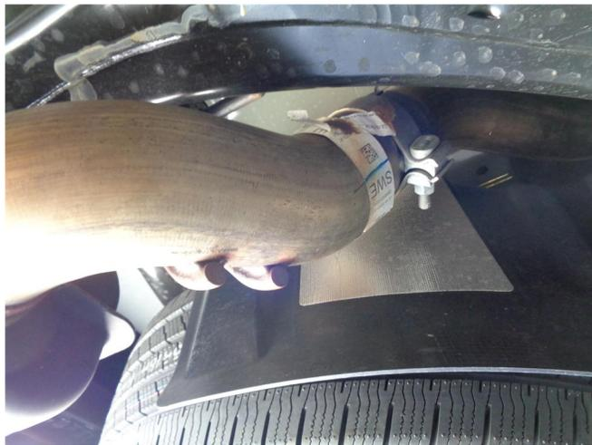
**Step 2.** Next, remove the tail pipe section by loosening the OEM clamp. Disengage the welded hanger from the rubber insulator and remove the tail pipe assembly. Do not discard or damage the rubber insulators as they will be used to mount the new system.
