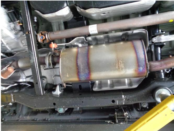
**Step 1.** To remove the OEM exhaust system you will first need to remove the rear sway bar.
