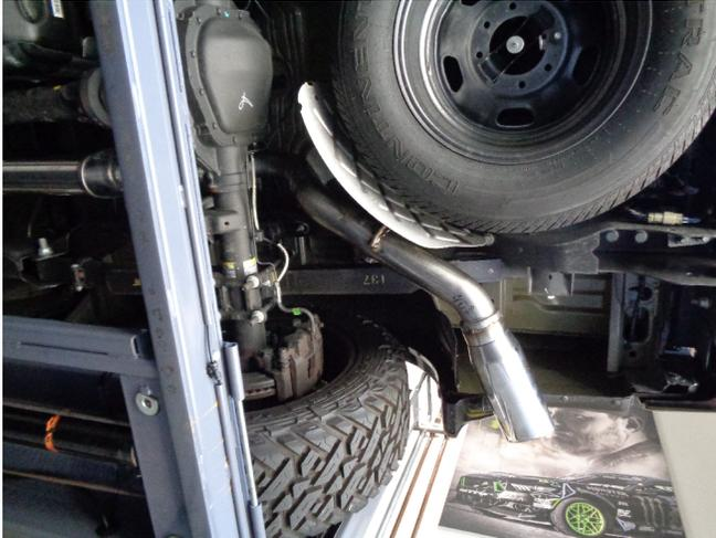
Step 6: Finish by loosely installing the Tail Pipe Assembly using the supplied clamp. Install the welded hanger to the rubber insulator.
