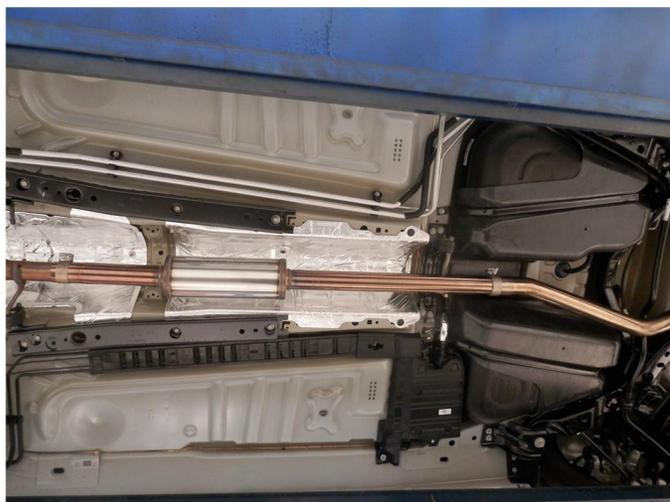
**Step 2.** Begin installation of the new system by fastening the Resonator Assembly inlet to the outlet of the catalytic converter using the supplied 2.25" band clamp. Please be sure to align the locating peg with the notch in the pipe. Leave all clamps loose for the final adjustment of the complete system.
