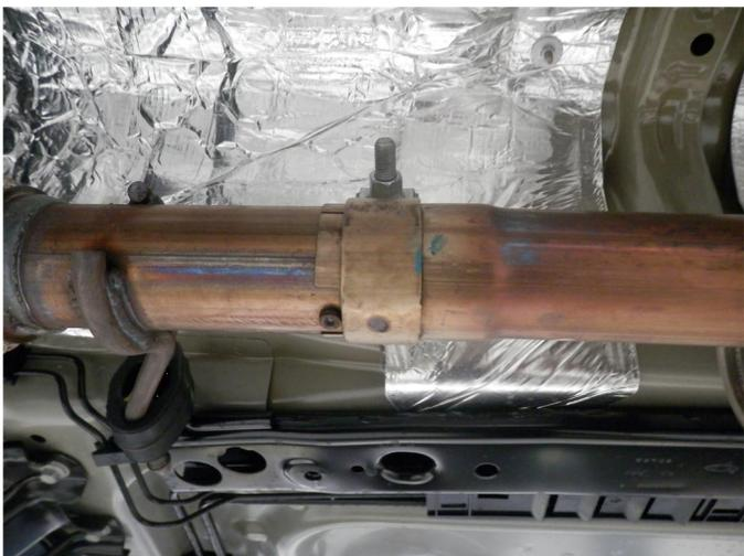
**Step 1.** To remove the OEM exhaust system loosen the clamp fastening the inlet pipe to the Catalytic Converter outlet. Working front to rear disengage all welded hangers from the rubber insulators and remove the system. Do not discard the or damage the rubber insulators as they will be used to mount the new system.
