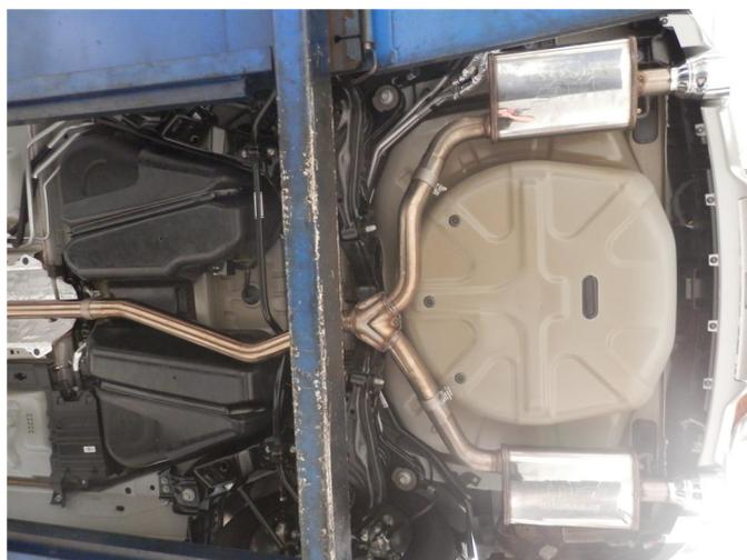
**Step 3.** Next loosely attach the Y-Pipe Assembly and both Muffler Assemblies using the supplied 2.50" clamps. Engage all welded hangers to the rubber insulators.
