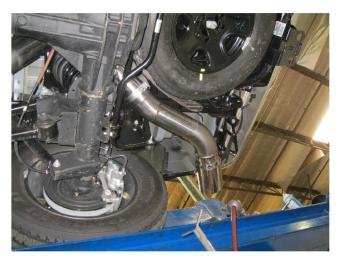
**Step 4.** Complete the installation by sliding the specified Rear Hanger Clamp Assy onto the Tailpipe Assy and attaching the Tailpipe Assy to the Over Axle Pipe. Engage the hangers into OE rubber insulators.
