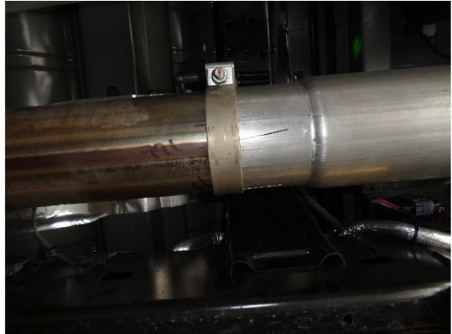
**Step 2.** Your vehicle configuration will determine which inlet pipe is used, see the table below. Begin installation of the MagnaFlow system by attaching the appropriate Inlet Pipe to the outlet of the DPF using the supplied 4.50" clamp.
