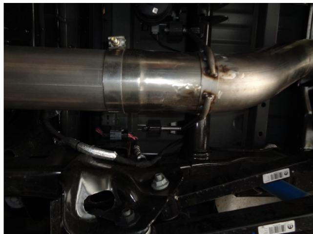
**Step 3.** Next, slide the Front Hanger Clamp Assy loosely onto the Over Axle Pipe Assy then attach Over Axle Pipe Assy to the Inlet Pipe using the supplied 5.00" Clamp. Engage the hangers into the rubber insulators. (Leave all clamp and fasteners loose for final adjustment of the complete system.)
