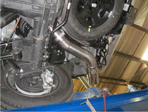
**Step 4.** Complete the installation by sliding the Rear Hanger Clamp Assy onto the Tailpipe Assy and attaching the Tailpipe Assy to the Over Axle Pipe. Engage the hangers into OE rubber insulators.
